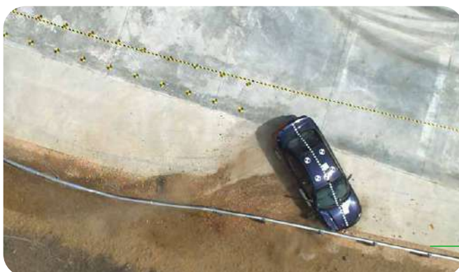
Crash test stand for testing barriers and supporting structures
